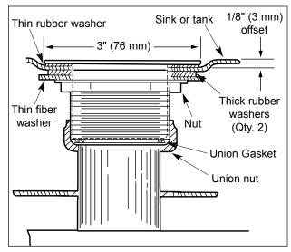
Figure 7. Installing Sink Strainer
